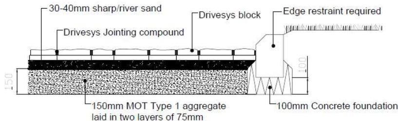
**\*\*Make sure rubber mat is used whilst vibrating the blocks, and also always vibrate prior to introduction of jointing compound\*\***
