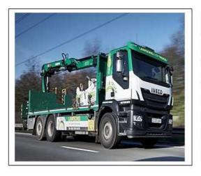
Leading the way we developed the first gas/electric 26 tonne HGV delivery vehicle alongside IVECO and Hiab. A key beneficiary, with the addition of this CNG vehicle to our operation, was the general public by way of the 50% reduction in noise, 99% reduction in particulant matter and 95% less CO2 when using biomethane. The second beneficiary of course is our driver who no longer has to operate the crane in a noisy, noxious environment.
