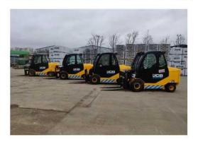
We collaborated with JCB in their development of an electric Teletruk and purchased the original demonstrator and the first four subsequent machines that went into production towards the end of 2019. Alongside our existing electric Combilift machines, this has resulted in the plant at our Edgware and Bedford branches being totally electric which again benefits our workforce by providing them with a cleaner, quieter working environment.
